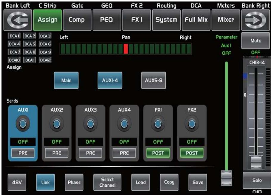
**Main** **AUX1-4** **AUX5-8** Touch Main, AUX1-4 or AUX5-8 on the LCD screen or corresponding button on the panel to assign input channel audio to these channels or buses. They will illuminate synchronizing with buttons in Assign area on the panel after pressed. To adjust output level of the channel audio, you can rotate Parameter Adjust knob or corresponding Main, AUX1-4 or AUX5-8 knobs on the panel.
