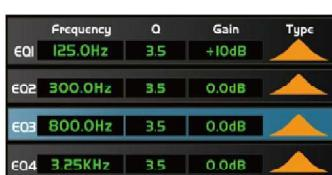
Touch EQ1 to set its Frequency, Q and Gain parameters separately, touch Type to change the filter to high-pass, low-pass or band-pass filter, the same as EQ2, EQ3 and EQ4. You can see the waveform on the screen.
