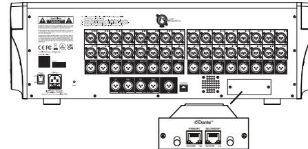
3). Insert the Module on the slots following the below picture and the Module must be on the middle of the slot.
